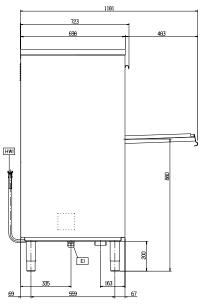
Drain EI = Electrical inlet (power) Electrical Outlet
